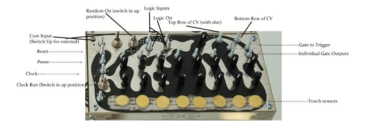
The 8x2 cv programmer is a classic fully analog cv programmer utility module. Yes, it has sequential functions but it's uses as a sequencer are rather limited to the point that certainly by today's standards I feel you can hardly even call it a sequencer. And viewing it as such in my opinion will most likely limit its usefulness.
